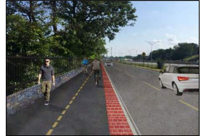
Top right: a stone wall and fencing treatment is proposed along the Yacht Club frontage. At a width of 8 feet, the path is less than the width of 10 feet recommended by AASHTO; a slight shift in roadway alignment could create the space needed for greater width, if desired. Below: trail along South Marginal Road.
