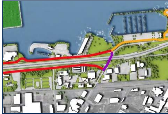
Top right: a stone wall and fencing treatment is proposed along the Yacht Club frontage. At a width of 8 feet, the path is less than the width of 10 feet recommended by AASHTO; a slight shift in roadway alignment could create the space needed for greater width, if desired. Below: trail along South Marginal Road.
