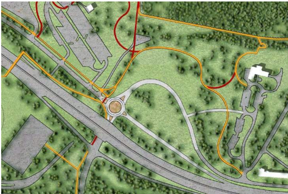
Top: MLK Drive existing conditions. Bottom: New paths are shown proximate to the Lakefront Nature Preserve. A roundabout is proposed to process traffic from westbound I-90 and Lakeshore Boulevard. This results in a smaller footprint for vehicular roadways than the existing loop road design.
